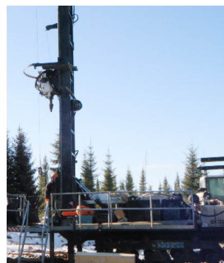
Mast head of a sonic drill rig. Sonic drilling proved very effective in sampling both overburden and rock material, defining 5 interesting diamond drill targets on the property.
