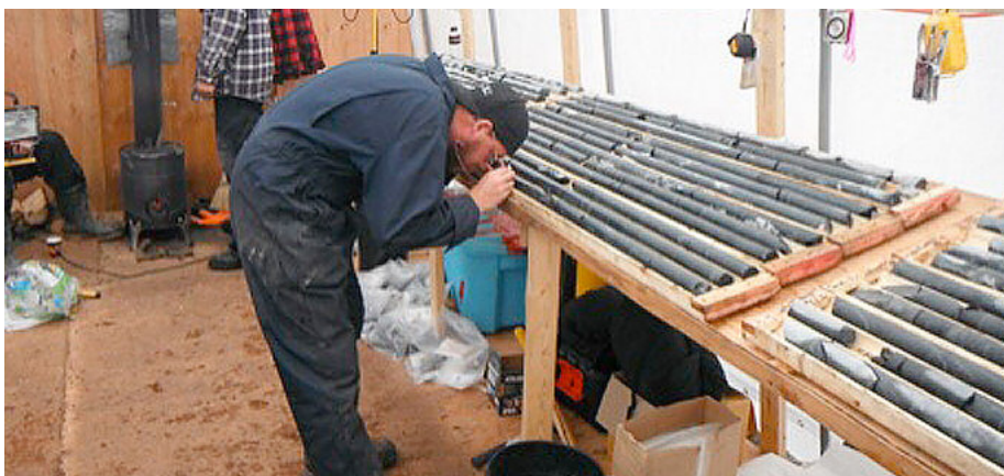
Drill core is processed on site. A Northern Superior geologist makes observations on drill core mineralization.
