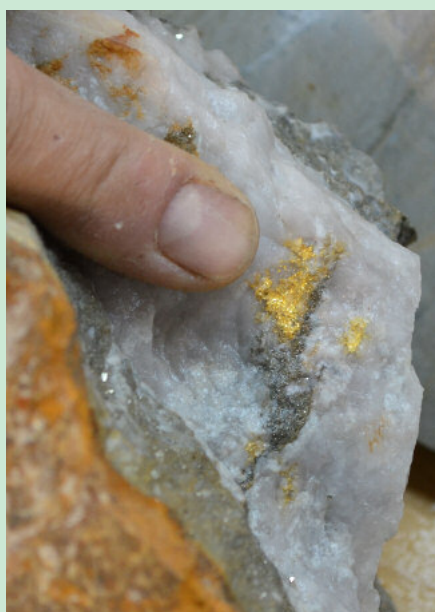
Coarse visible gold (gold colored flakes) in fly rock from Trench 3.
