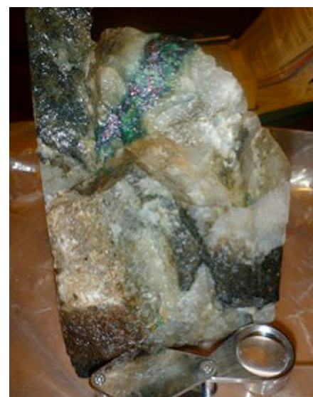
Quartz veins hosted in highly sheared monzonite containing bornite-chalcopyrite with 2-3% disseminated fine-grained arsenopyrite.
