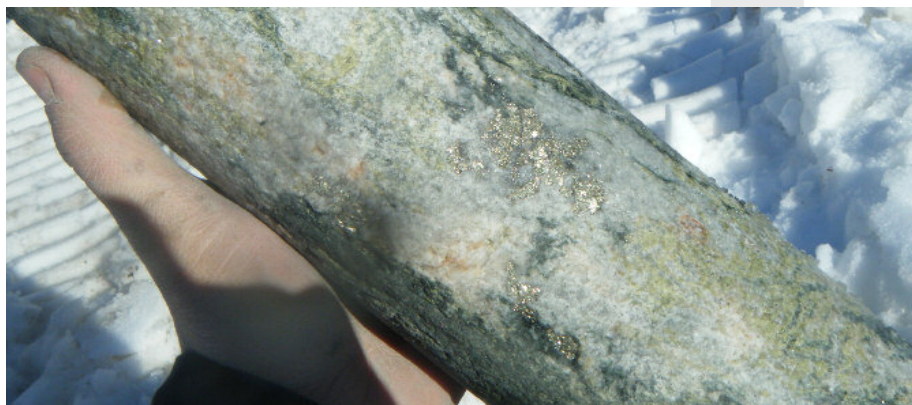
Sonic bedrock core. Core consists of mineralized sheared material associated with the Kapunapotagen Fault that trends east-west, passing across both the Chibougamau River and Lamarck Creek Faults.
