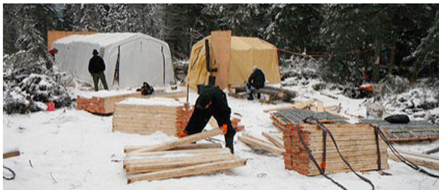
Drill core processing facility. Core is transferred from the drill site to this facility where it is logged, sampled and packaged for shipment to a laboratory for assay work.
