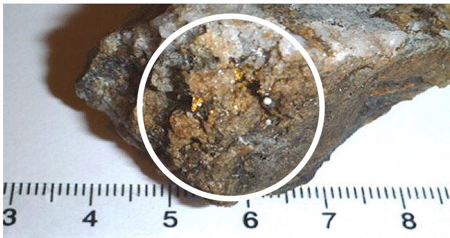
Part of a large (2 x 3 m) boulder containing coarse visible gold (gold mineral circled in white).
